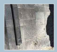
The MIB<sup>2</sup>S block defeated 126 rounds of .50 Cal BMG API fired in rapid succession from 50 feet in manufacturer testing (The MIB<sup>2</sup>S pictured below)
